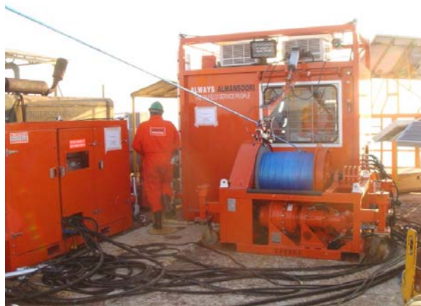
Figure 1: Pulling Rope and Winch
