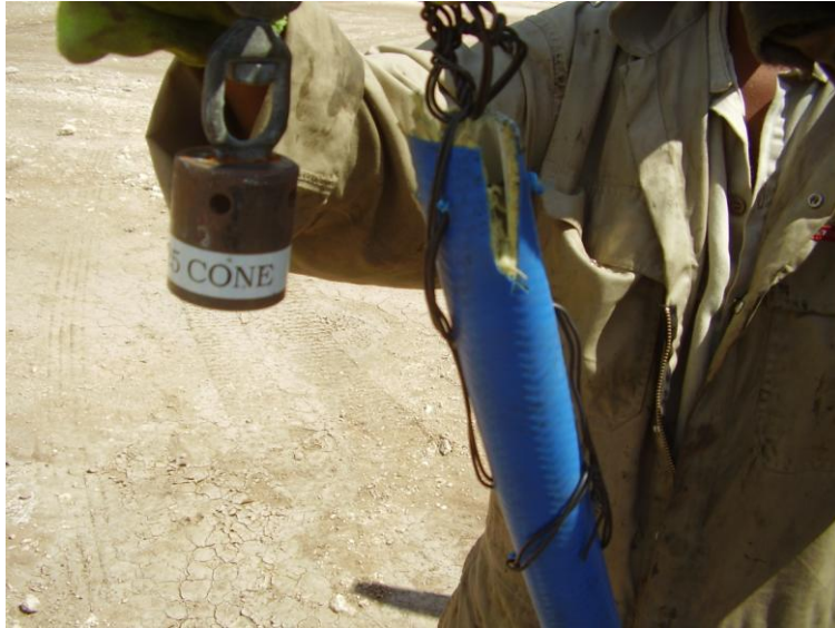
Figure 3: Pulling Cable compared with the Pulling Cone
