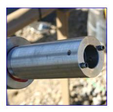
The pump discharge head is equipped with a break away fitting for in case the pump and tubing gets blocked during insertion in the well.
